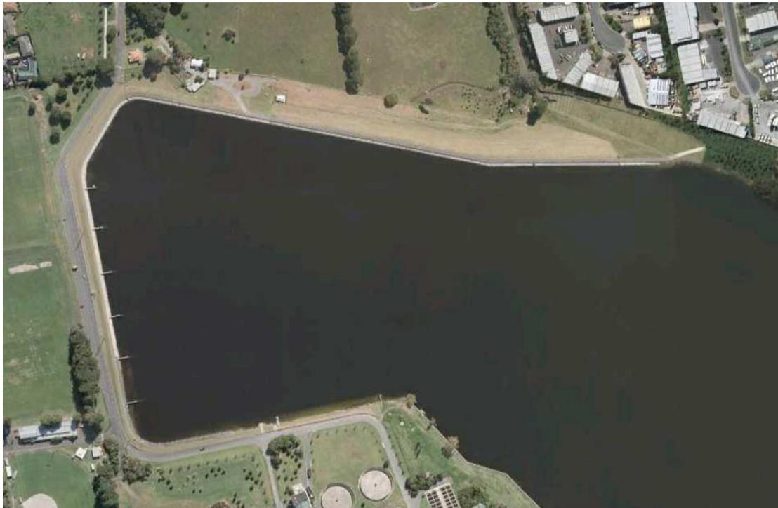
The total embankment is approximately 1 km long, and retains approximately 1,750,000 cubic meters of treated wastewater.
